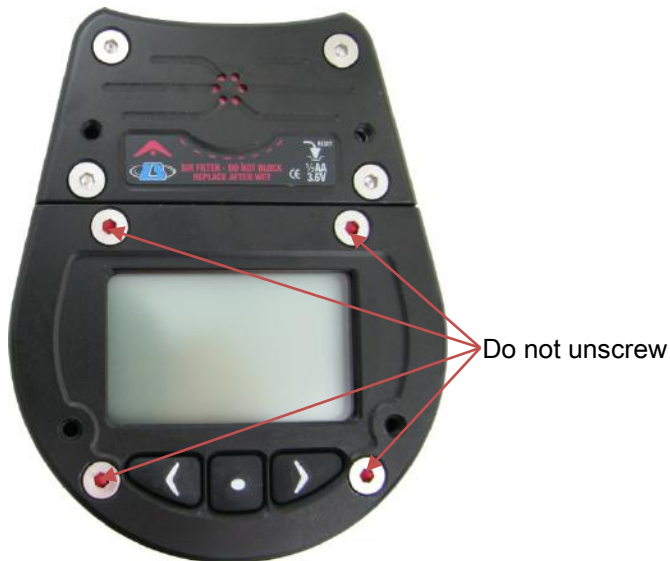
Fig. 23 - Note: Four sealed screws must not be removed.
