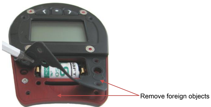
Fig. 25 - Pay attention that the surfaces underneath and on the black rubber sealing are clean.
