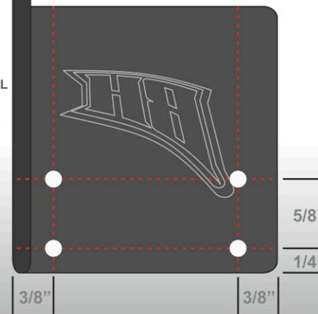
3. Using the 1/8" drill bit and drill, drill holes where the dimension lines cross.
