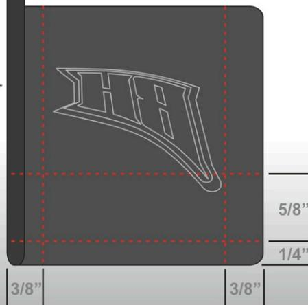
2. Measure out the above dimensional grid to determine slot and drilling placements.
