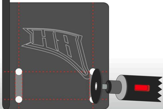
4. Use a Dremel or Rotary tool to remove the material in between the holes. Be careful and go slow.
