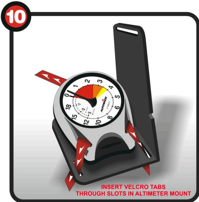
INSERT VELCRO TABS THROUGH SLOTS IN ALTIMETER MOUNT
